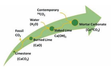
Fig.1: Basics of mortar production
