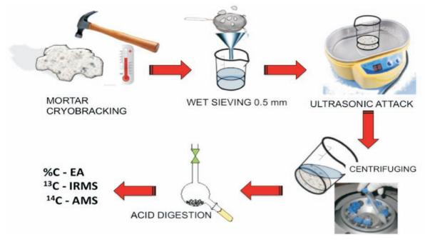
Fig.2: New protocol for mortar preparation
