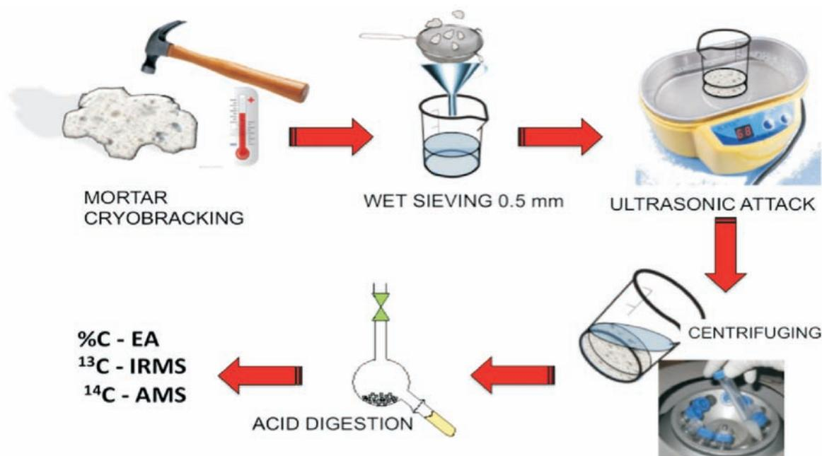
Fig.2: New protocol for mortar preparation
