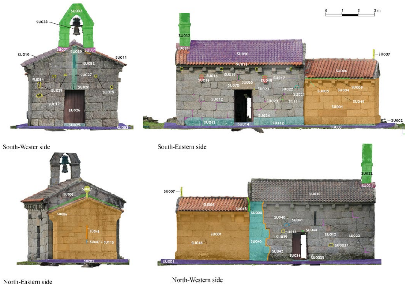
Figure 5. View from outside the church of the various walls with relative indications of the SU. Digital processing by authors.
