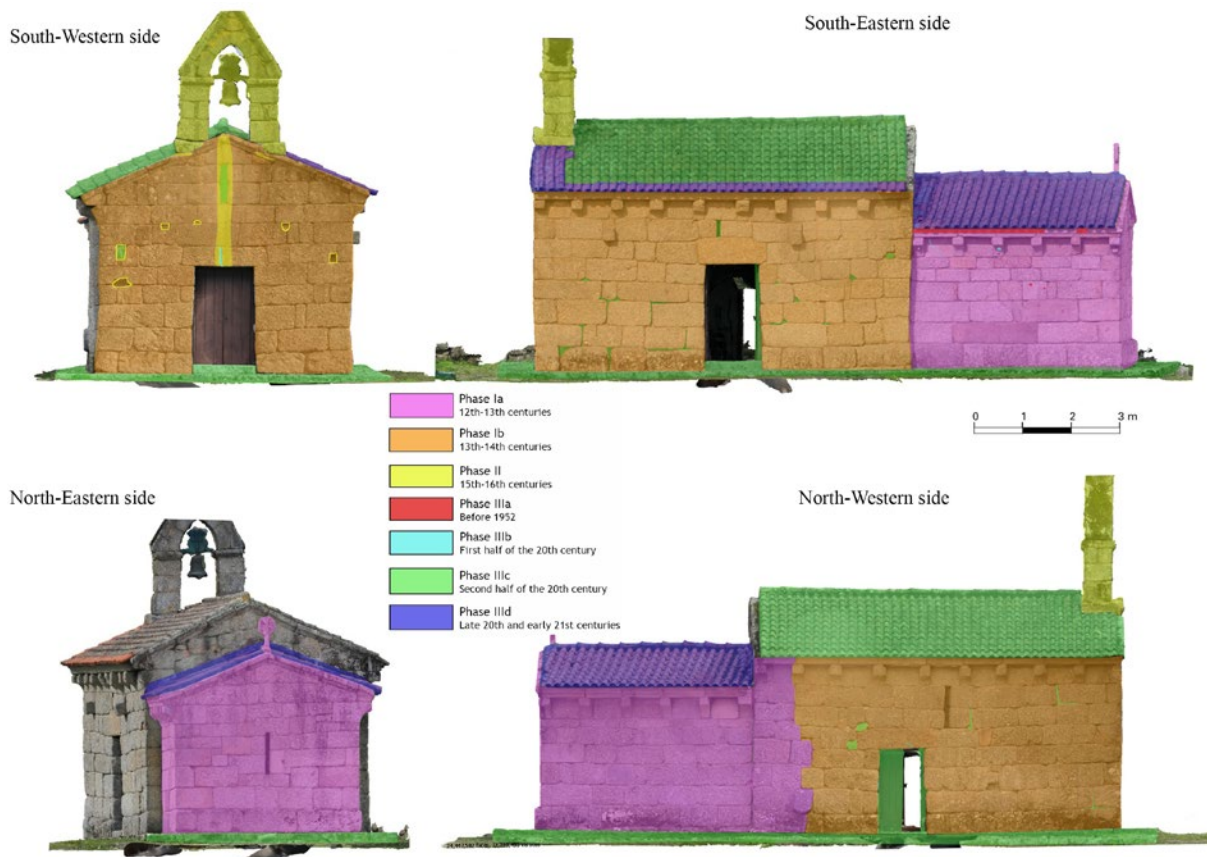
Figure 8. View from outside the church of the various walls with relative indications of the construction phases. Digital processing by authors.
