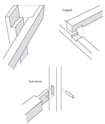
Fig. 2. Basic joints attested from excavated waterlogged timbers include lap, cogged and tusk tenons.
