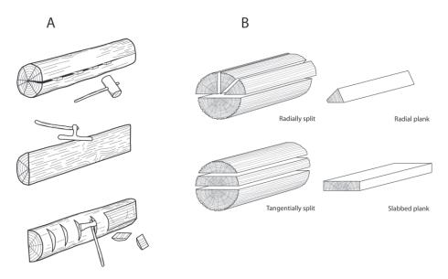
Fig. 3. A. Timber could be prepared in the early Middle Ages by splitting radially or tangentially. Once the timbers had been split to size, they were be finished by hewing (or trimming) the faces with a T-shaped axe and, where necessary, by removing the waste by notch-and-chop hewing (after Hill and Woodgar 1999, 49). B. Radial and tangetial planks.
