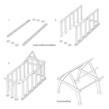
Fig. 7. The method of construction used in the early medieval tradition identifed here may be contrasted with cruck construction which though suggested by a number of archaeologists is not attested before the thirteenth century.
